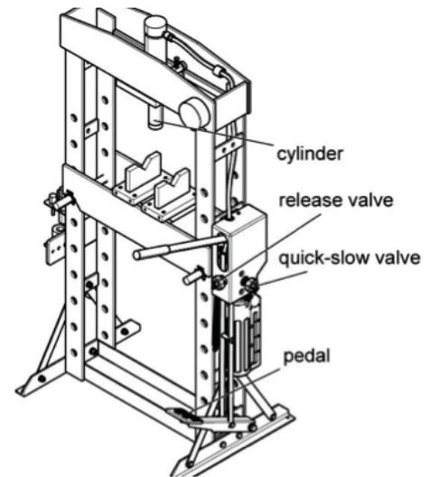
2. Please conduct the following operations to discharge the air out of the hydraulic system, when finding the slow function of the hydraulic pump is not working or the pump can't load pressure during using (especially for the first time).
